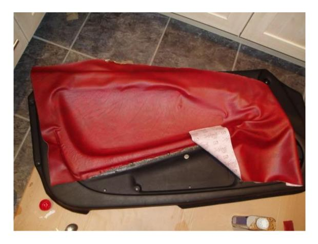
I DIDNT GLUE RIGHT TO THE EDGE OF THE DOOR CARD TO WHERE IT DIPS INTO THE DOOR - I LEFT THIS TO THE END THEN WENT ROUND WITH SCISSORS AND A SMALLER BRUSH - THIS MAYBE WHERE I WENT WRONG! MY EDGE WAS QUITE TATTY AND I TOTALLY DESTROYED ONE PART BY USING LOCTITE - WHEN IT COMES IN CONTACT WITH THE A29 IT MELTS THE LEATHERETTE!!! SO YOU'LL HAVE TO FIND YOUR OWN WAY WITH THE EDGING - UNLESS YOU'RE PLANNING ON FITTING A TRIM LIKE MY CHROME ONE.
