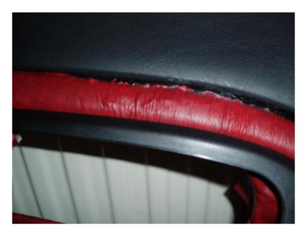
AREA 5 IS EASY ALTHOUGH YOU HAVE TO WORK SLOW AND CAREFUL TO GET A NICE FINISH. MAKE SURE YOU'VE TRIMMED THE EDGE SO IT'S ALMOST TOO SHORT BECAUSE THE VINYL WILL STRETCH WHEN YOU PUT THE GLUE ON IT AND YOUR EDGE CAN END UP ALL UNEVEN.
