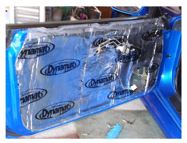
10. REFIT THE SPEAKER AND CONNECT UP. DON'T WORRY ABOUT THE SCREW HOLES THE SCREW SHOULD PUSH EASILY THROUGH THE MAT AND INTO THE DOOR.
