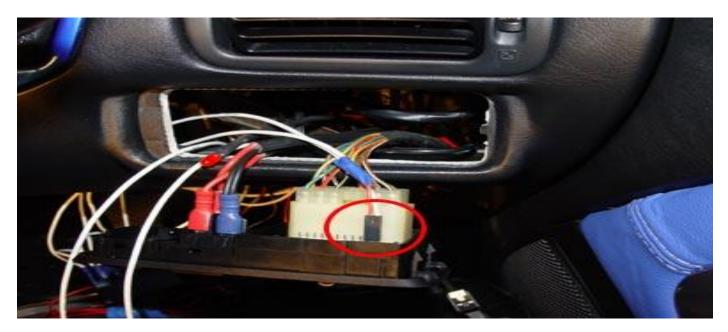
Remove the mirror control panel, lift up the black plastic cover to reveal the pin connectors and attach the open and close signal wires to the two rightmost pins. I used a pin connector from an old PC case instead of messy soldering here. Test the central locking and if the mirrors fold incorrectly (ie. fold out when car is locked then simply swap these two connections around.
