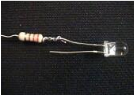
RESISTOR CONNECTED TO POSITIVE LEAD.
