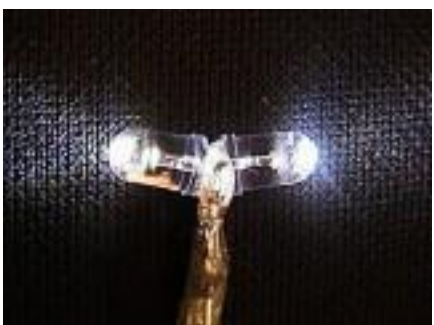
LED BULBS SOLDERED & THEN GLUED TOGETHER.
