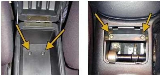
Once removed the centre console can come up, and away exposing the handbrake cable, the lever bracket, and the plunger switch. See below:
