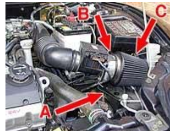
A: Support B: Adaptor C: Filter
