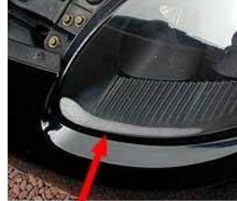
Fog on the inside of the light Metal rod stuck thru into light
