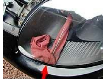
Cloth stuck into light thru the main beam bulb hole.
