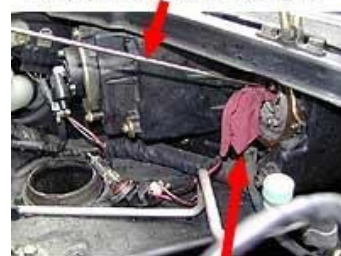
Cloth sticking out - make sure you don't lose the end inside the light
