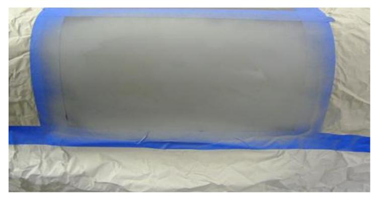
To further prepare and protect your repair, you'll spray the surface with a primer/sealer. Mask off an area around the repair to avoid getting paint on any trim or other non-painted areas (don't forget, you don't want paint on your tires, either). Apply the spray primer in light, even coats. Three light coats are better than one heavy coat.
