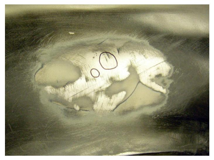
Before you can fill your dent, you'll need to remove the paint. Body filler doesn't stick well to paint, so you need to sand it down to bare metal. For this job, you can use a heavier grit sandpaper like a 150-grit. You want to get the paint off fast, and you'll be smoothing things out later anyway.
