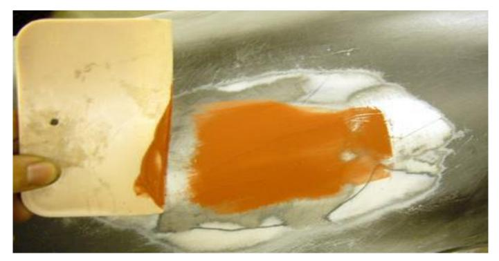
Spot putty is another version of filler, but much finer and easier to sand. It doesn't need to be mixed and can be applied directly from the tube to the repair. The spot putty fills in any tiny impressions in the filler.
