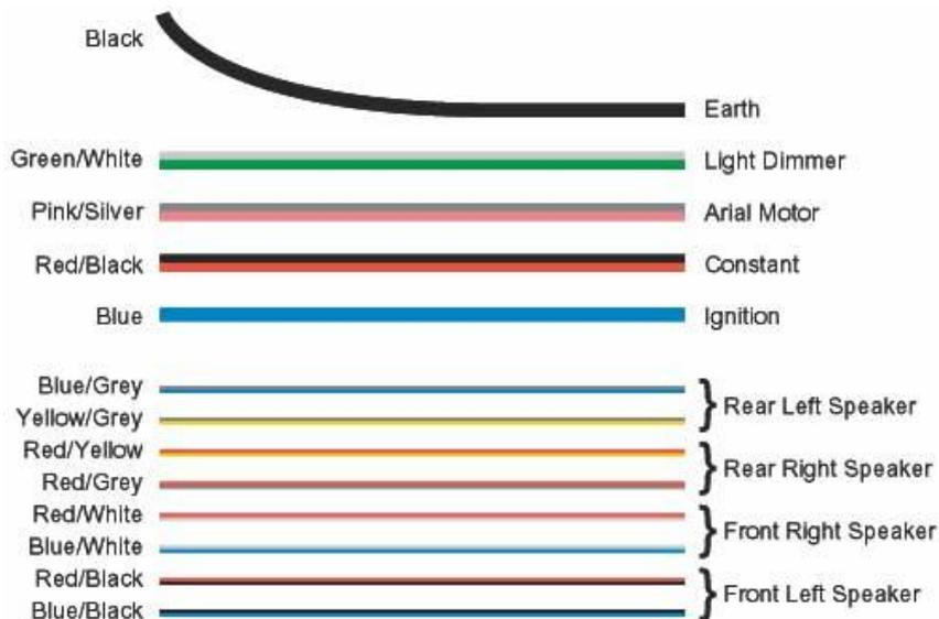
**Important:** There is no direct earth wire in the FTO stereo loom. You need to connect a new wire to earth. If you don't do this you risk blowing fuses and random lights/arial/no-constant problems!
