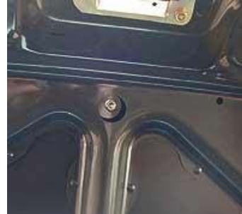
The bolt in the middle, holding the centre strut
