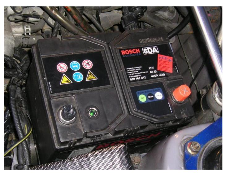
FIRST OFF YOU WILL NEED TO CHANGE THE TERMINAL CLAMPS AS THE OEM ONES ARE TOO SMALL. I BOUGHT SOME FROM HALFORDS FOR UNDER £10. BE CAREFUL WHEN BUYING TO GET BOTH 'P' AND THE 'N' TERMINALS AS THEY ARE DIFFERENT SIZES!!
