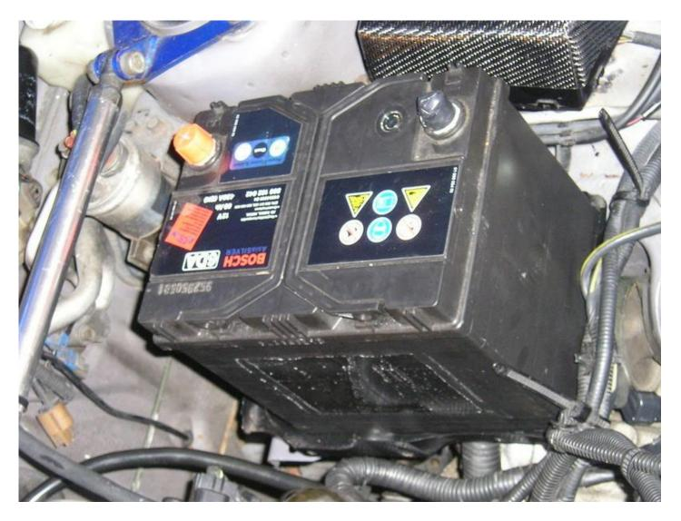
THEN THE CLAMP WILL NOT FIT THE NEW BATTERY, AS THE CLAMP IS TOO NARROW MODIFIED MINE BY HACKSAWING A BIT OF AND THE BENDING THE CLAMP FLAT LIKE THIS
