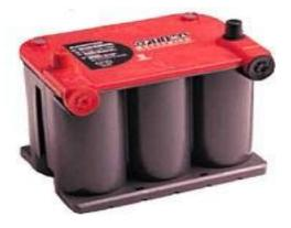
Dimensions: 9.313" Long x 6.813" Wide x 7.625" Tall Weight: 33.1 lb (15.0 kg) Power: CCA (BC10°F) 720 amps, MCA (BC32°F) 910 amps Capacity: 44 Ah (C/20) Reserve Capacity: BCI 90 minutes (25 amp discharge, 80°F (26.7°C), to 10.5 volts cutoff)
