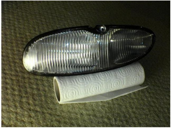
With this done its time to put the new silver bulbs in (you can get these off ebay for about £5 Opposite Pin Indicator Bulbs) Then replace the wiring harness and put them back in the bumper. Job done.. I hope this helps.
