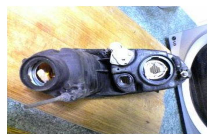
Next comes the scary part. You are going to bake the unit in the oven for 5 mins or so to loosen the glue holing the 2 halves together.
