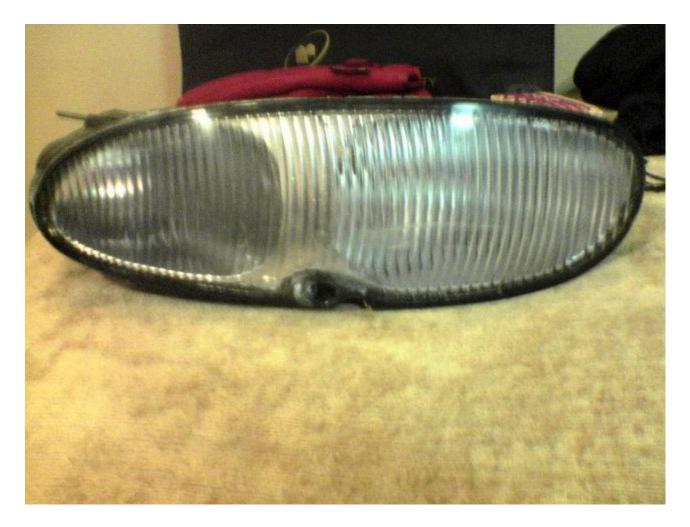
I found at this point that they did not seal all the way around and thought it best if I used an epoxy to replace the glue that was lost. I just used a 2 part epoxy, mixed it together and went around the joint between the light and the housing till there was no more gapes. Dont forget to wipe off any glue you get where you dont need it.
